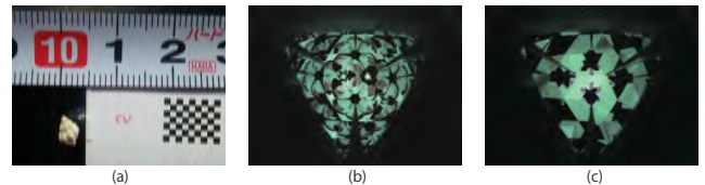
Fig. 32 Teleoscopic imaging. (a) Captured object (approximately 5mm size). (b) Image by our system. (c) Image Without the monocentric lens. The refraction by the monocentric lens provides the surround view.
