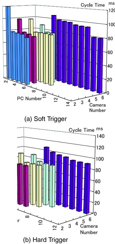
Figure 7: Overall computation time for reconstructing one 3D shape measured by changing the numbers of cameras and PCs.
