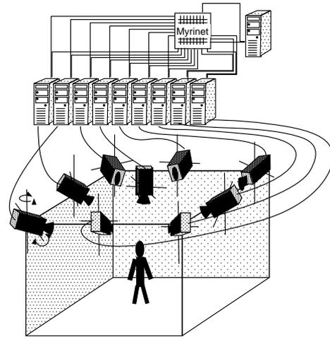
Figure 2: PC cluster for real-time active 3D object shape reconstruction system.
